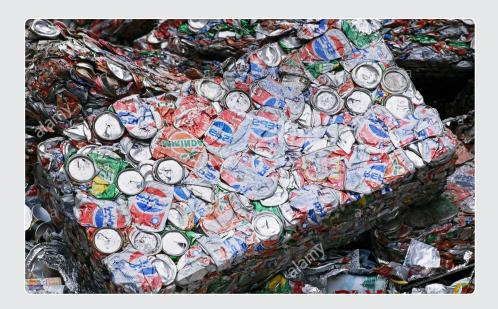
Baling is particularly common for paper and cardboard due to the large volume they take on site. Baling also takes place typically for plastics and cans. The dimension and weight of the bales shall be designed to meet the end market requirements in terms of export and container cargo sizes.
